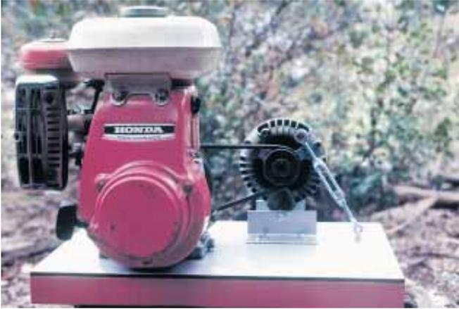
Above: The engine powering this generator is a Honda G40 model displacing 170 cc with a rated output of 4.5 horsepower. This particular engine has outlived four alternators and now powers a 100 Ampere Chrysler alternator. I estimate that this engine has run over 13,000 hours in the last fifteen years. It still has its original valves and piston rings.
